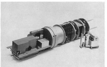
COMPACT INSTRUMENTATION PACKAGE for the Zero G facility is 32 inches long, five and one half inches in diameter, and weighs 35 lbs. Left is 16-mm movie camera. Right is tape recorder.
